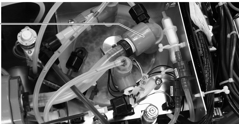
Figure 5.135 Vacuum elbow location, 5122
