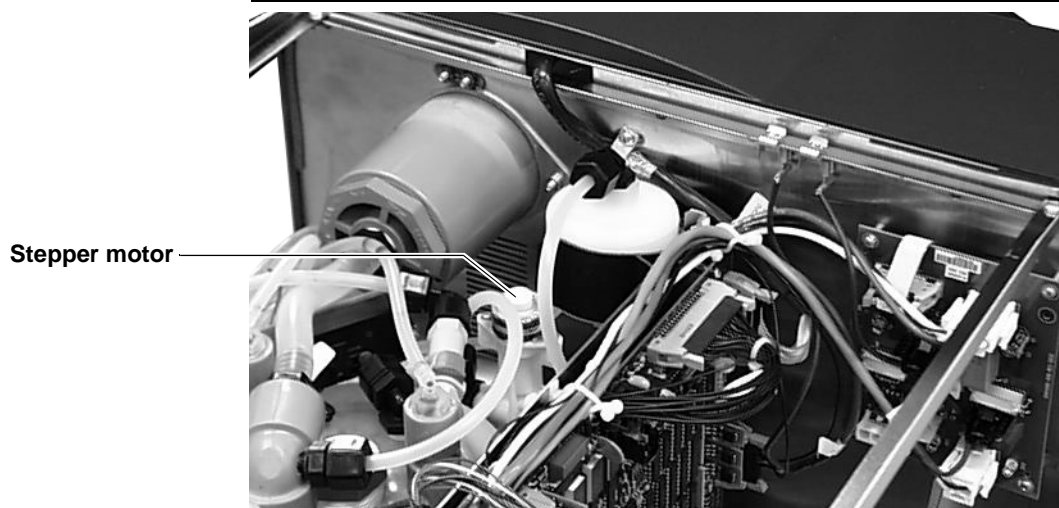
Figure 5.133 Stepper motor location, 5122
