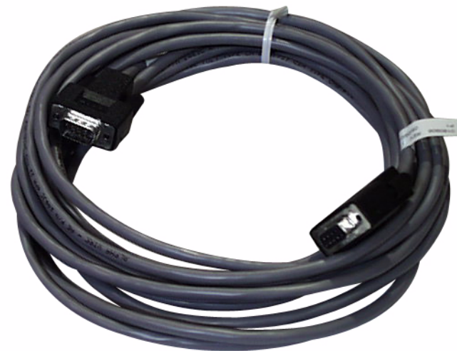
Figure 5.240 Tach and cue extension cable, 20-ft. (0183205)
