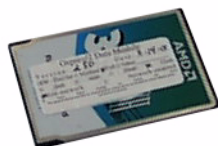
Figure 5.72 32-MB flashcard (0179654), V2.30 and standard US fonts
