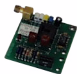
Figure 5.199 Tab buffer board (0178591), 5120 printhead
