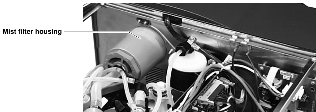
Figure 5.127 Mist filter housing location, 5122
