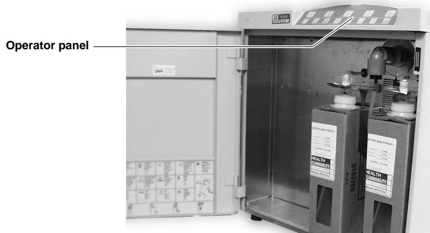
Figure 5.47 Operator panel location, 5122
