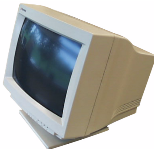
Figure 5.226 Monitor, 14" viewable screen (0104004-030)
